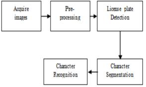
Fig 1. Block diagram of License Plate Recognition System
